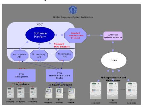
Each manufacturer provides its own encryption / decryption API, integrated into the system software.
